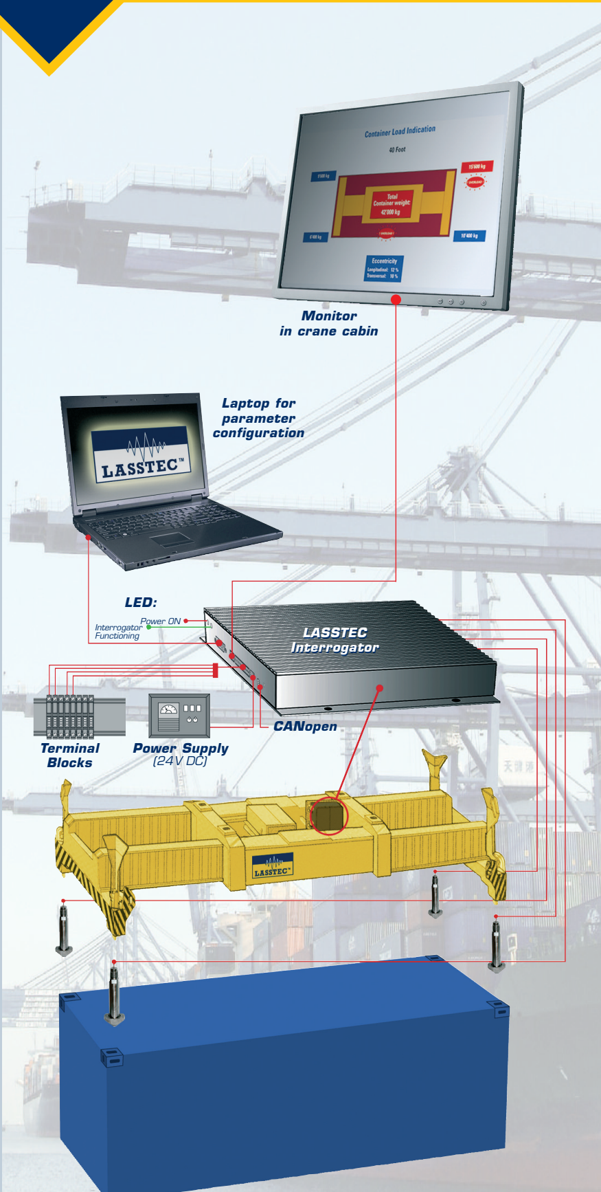
Twistlock sensors in each corner of the container capture and send valuable, individual load data to the Interrogator (data processing unit). Data is analyzed, and output signals are fed to the crane PLC and displayed on a monitor in the crane cabin.
